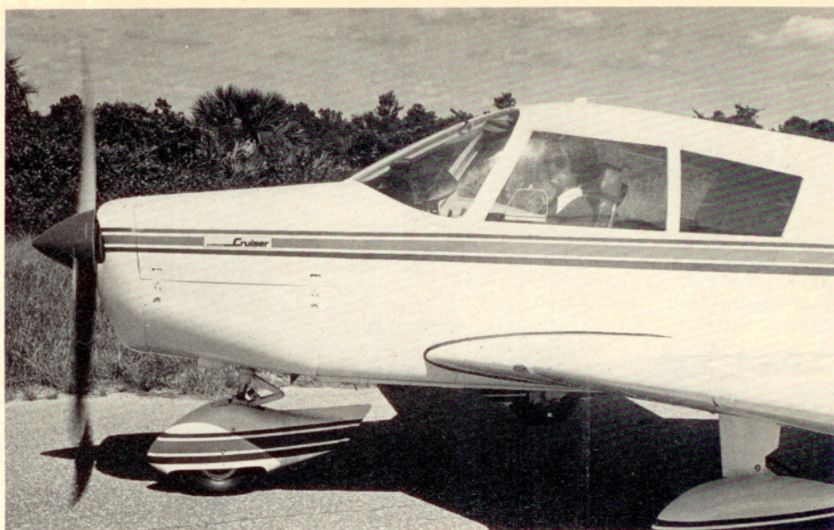
By applying techniques to minimize structural shock to the nosewheel, the pilot can reduce the likelihood of the embarrassment—and cost—of a collapsed gear.
